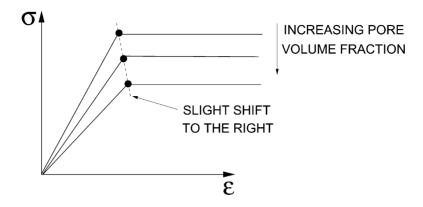
Figure 1: Idealized stress-strain curve.
