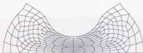
Figure 2: Compression of a rubber block (a) result of a locking-free element formulation
